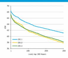
The above shows the top 300 hours of load for 2011, 2012, and 2013 YTD
